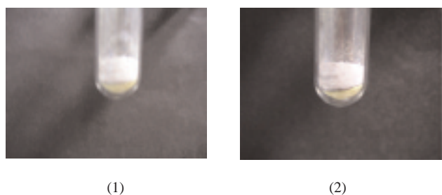
Fig.2 Change in state of two-layer of acridine and 3-methyl-1-phenyl-5-pyrazolone: (Upper part: 3-methyl-1-phenyl-5-pyrazolone, Lower part: acridine.) (1) initially; (2) after heating for 5hr at 50°.
